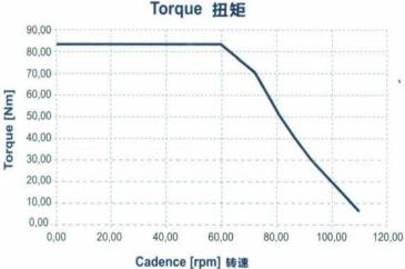
The driving torque shows that the motor is designed to deliver a maximum thrust up to a cadence of 60 rpm, while maintaining a high motor output even at higher rotational speeds. The power of a motor is calculated by multiplying the torque by the angular rotational speed. As a result, as the cadence increases, the power increases to a peak point that allows cyclists to reach their maximum riding speed (which is however limited to 25 km/h as required by law).
