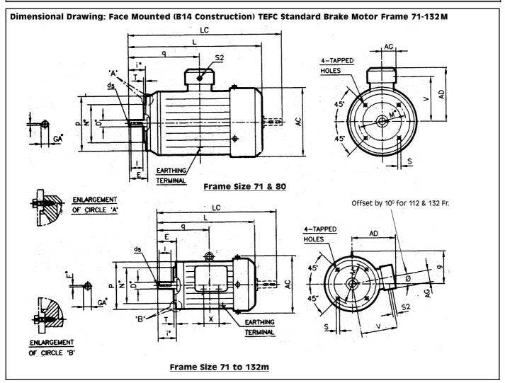
Dimensional Details: Face Mounted (B14 Construction) TEFC Standard Brake Motor Frame 71-132M
