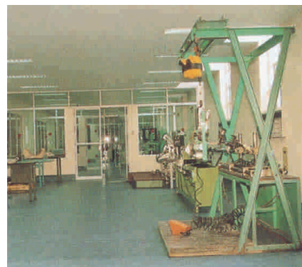
Air-conditioned dust free facility provided for coil making and insulation taping.
