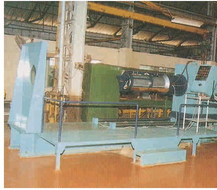
Core Insertion Machine installed for insertion of wound core into frame.
