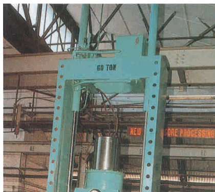
Vertical press installed for accurate rotor core building.
