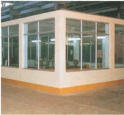
Dust free facility installed for Motor winding.
