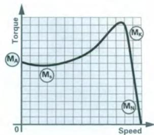
During the run up period in Star, there must be an adequate excess of motor torque over the load torque. The change to Delta must not occur until the motor is near the operating speed. Refer to Brook Crompton for running up against a load in excess of 70% full load during Star Delta starting.
